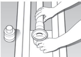
2 Install waste & screw ply to battens
